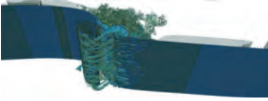
图2 波浪破碎中水气泡混合流生成与涡丝的数字模拟结果 [17] Fig.2 Numerical simulation results of water-air-bubble mixed flow generation and vortex filament in wave breaking [17]
