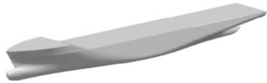
图3 KCS船模船体视图 Fig.3 The KCS ship model
