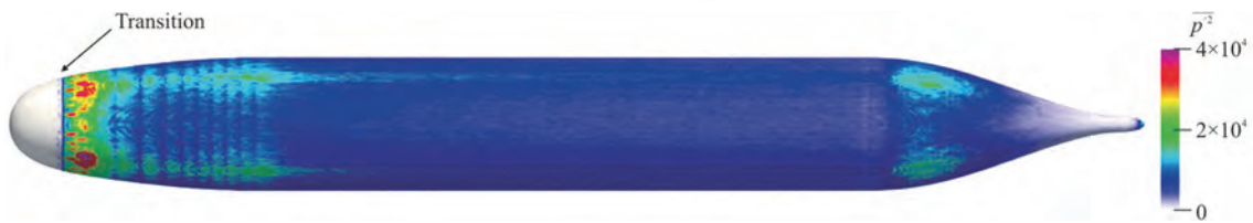
Fig. 12 (Color online) Time-averaged square of the pressure oscillation on the hull
