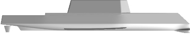
Fig. 2. Geometry model of ONR Tumblehome ship.
