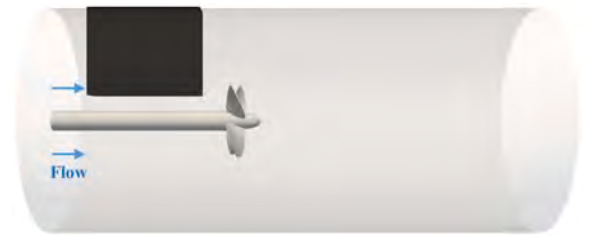
Fig. 2. The artificial non-uniform wake generator for INSEAN E779A propeller.
