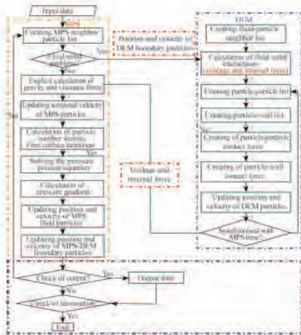
Fig. 3. Flow chart of MPS-DEM for two-phase flows.
