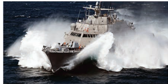
(a) Bow wave breaking and water-air-bubble mixed flow generated by high-speed warship
