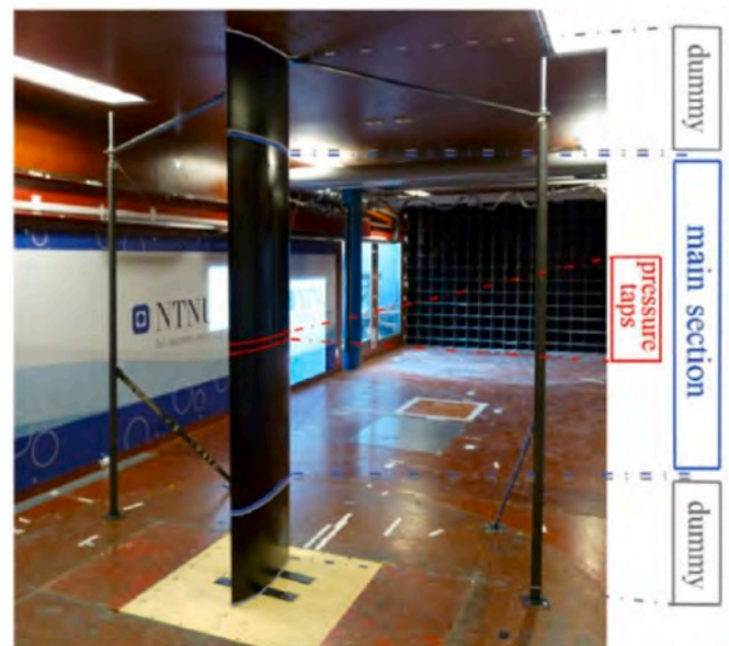
Fig. 2. Experimental configuration of the NREL S826 airfoil wing section test, adopted from (Bartl et al., 2019).
