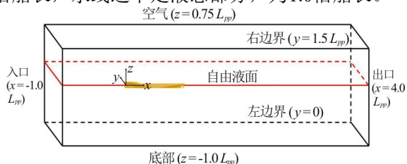
图2 (网上彩图)计算域与坐标轴设置 Fig.2 (Color online)Computational domain and coordinate axis set
