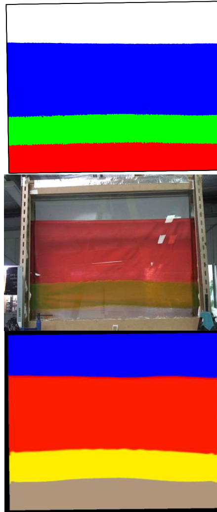
Figure 3 Snapshots of harmonic roll motion (zero degree) at 1.83 rad/s. Present method (top), experiment (middle) and simulation (bottom) of Molin et al. (2012). Upper layer-cyclohexane, middle layer-water, lower layer-dichloromethane.
