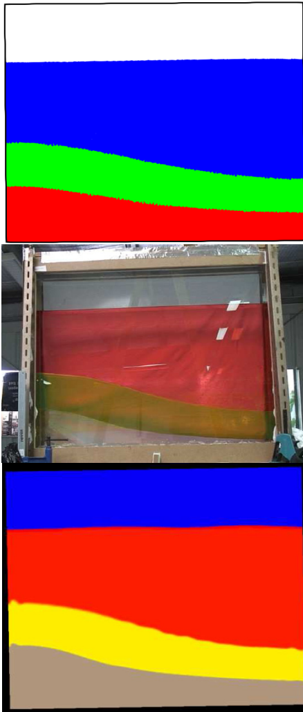
Figure 2 Snapshots of harmonic roll motion (maximal degree) at 1.83 rad/s. Present method (top), experiment (middle) and simulation (bottom) of Molin et al. (2012). Upper layer-cyclohexane, middle layer-water, lower layer-dichloromethane.
