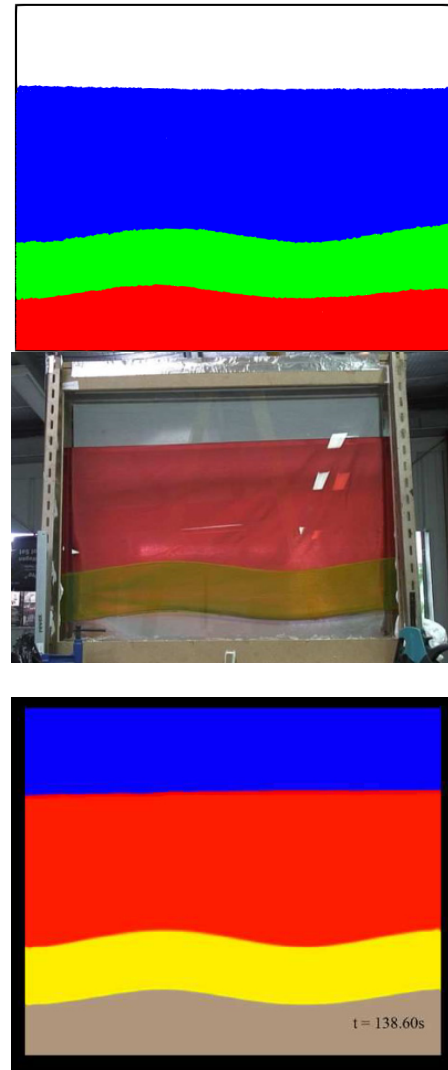
Figure 6 Snapshots of harmonic sway motion at 3.62 rad/s. Present method (top), experiment (middle) and simulation (bottom) of Molin et al. (2012). Upper layer-cyclohexane, middle layer-water, lower layer-dichloromethane.
