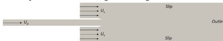
Figure 6 Boundary conditions of case with ambient flow.
