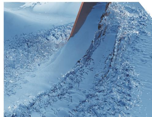
Fig. 3 (Color online) Long bubbly wakes behind the plat (flow field is rendered with ray tracing technique)
