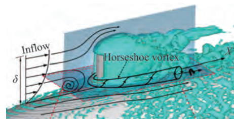
Figure 36 Horseshoe vortex behind the sail (Qu et al., 2021)
