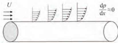
Figure 9 Fully developed axisymmetric turbulent boundary layer flow with high Reynolds number and zero-pressure-gradient over the midbody
