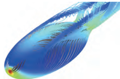
Figure 5 Crossflow transition around an ellipsoid (Israeli Computational Fluid Dynamics Center, 2014)
