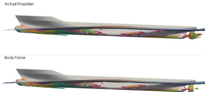
Fig. 12 Vortical structures around ship hull (upper: actual propeller, lower: body force propeller)
