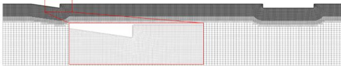
Figure 2. Mesh for the 2D flat-plate numerical simulation.
