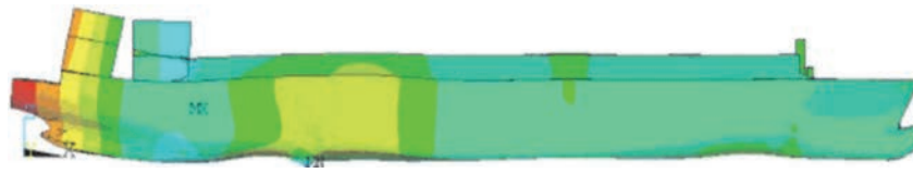
Fig. 10 (Color online) Hull girder modes at eigenfrequency of 3.59 Hz for wave [103]
