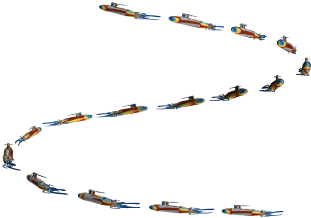
Fig.10. Vortex distribution and trajectory characteristics of the submarine space spiral maneuver.
