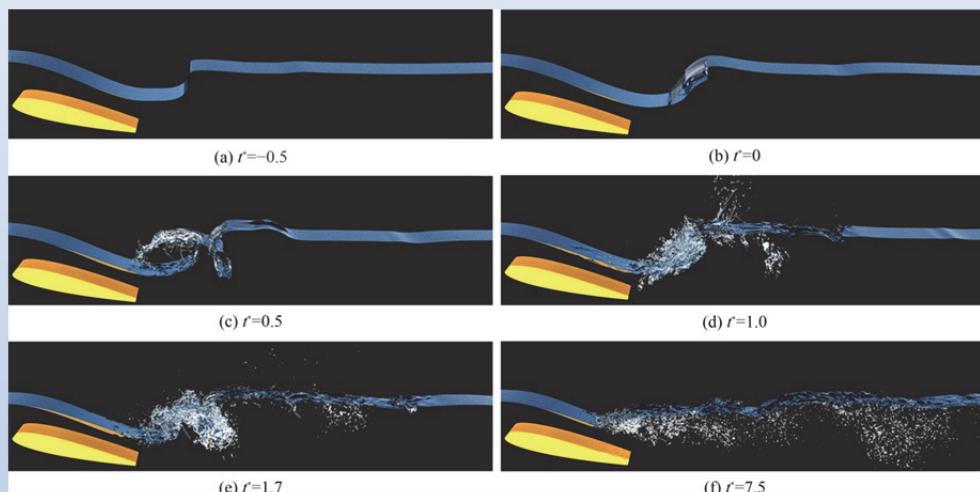
Numerical simulations of breaking waves generated by a 3-D submerged hydrofoil
