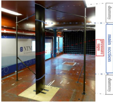
Figure 2 Schematic of the model experiment at NTNU [Bartl 2019]
