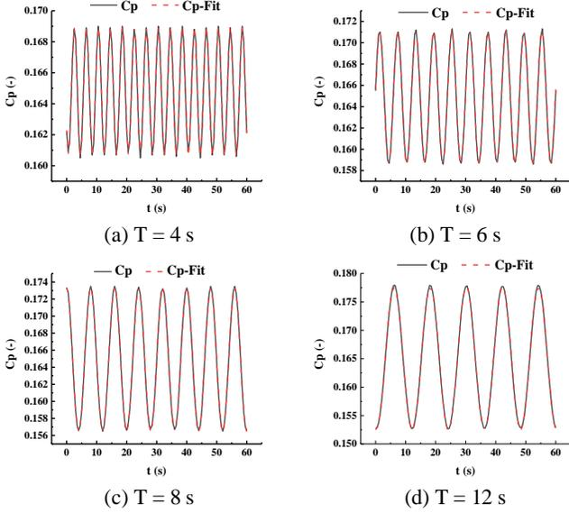
Fig. 9 Energy utilization coefficient fitting curve
