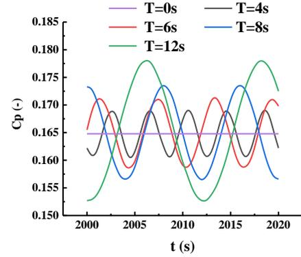
Fig. 4 Energy utilization coefficient time history curve
