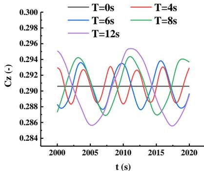
Fig. 3 Axial load coefficient time history curve
