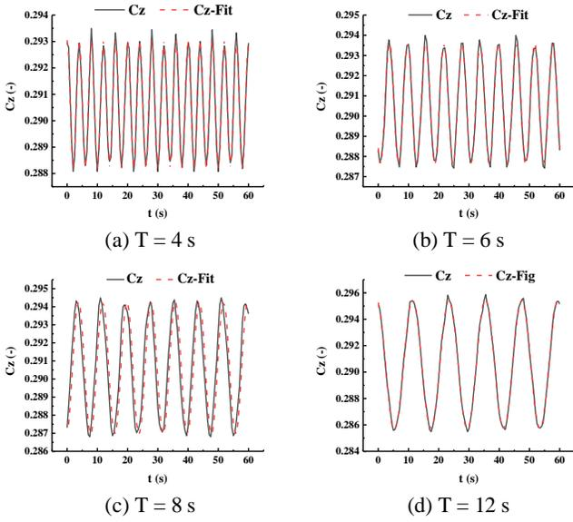
Fig. 8 Aerodynamic load coefficient fitting curve
