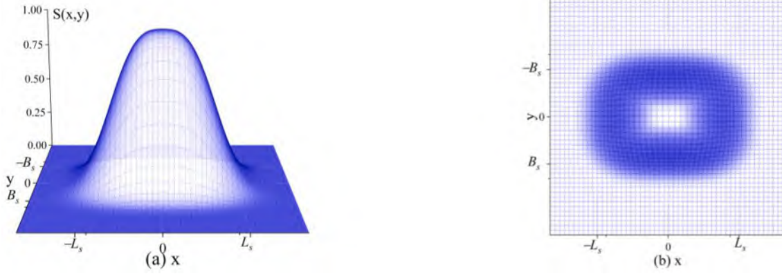
Fig. 1. Schematic diagram of the Gaussian pressure distribution described by Eq. (15), where n_x = n_y = n = 3 and \beta_x = \beta_y = 2^n \log(a) , a = 7.39 (the value of a is same as which in Lo (2021)). (a) Three-dimensional view; (b) top view: the central white area shows the characteristics of the platform.
