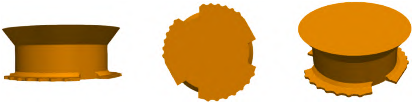
Fig. 1. Geometric model of the FPSO (a) Side view; (b) Bottom view; (c) Perspective view.
