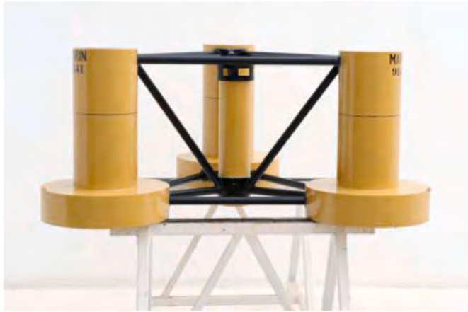
Fig. 2. Demonstration of the DeepCwind semi-submersible platform (Robertson et al., 2017).
