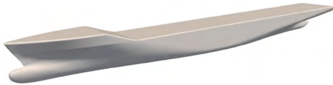
Fig. 9. Geometry of the KCS ship.
