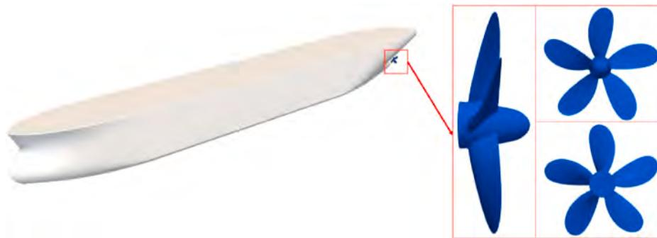
Fig. 6. The model of hull and propeller.
