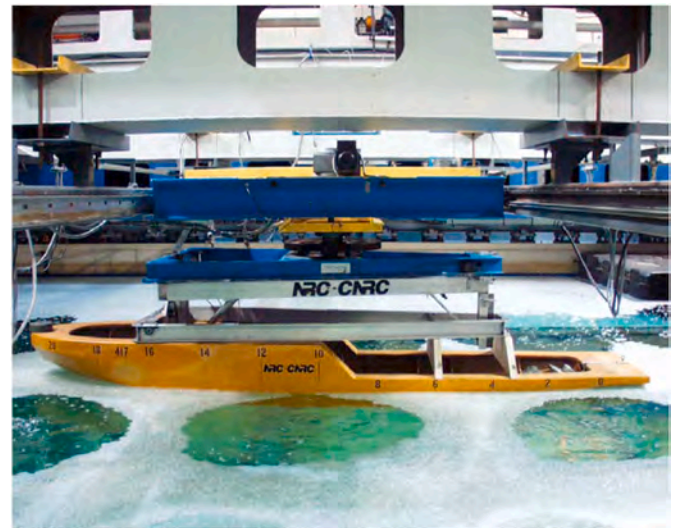
Fig. 3. Planar Motion Mechanism (PMM) test setup (Derradji-Aouat and Thiel, 2004).
