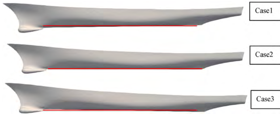
Fig. 5. DTMB5415 geometry under different sailing attitudes.
