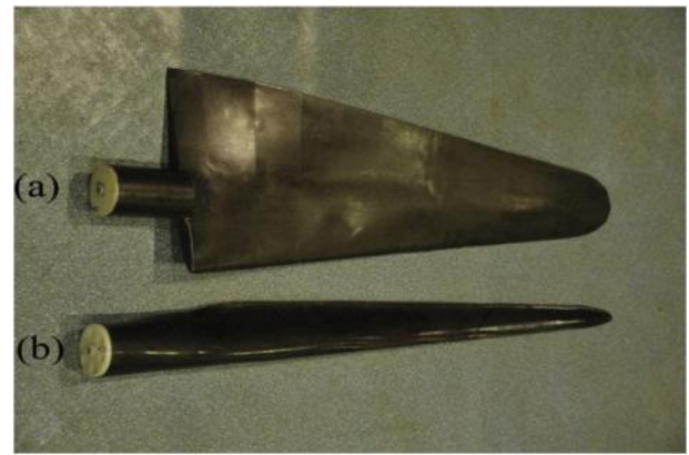
Fig. 2. Comparison of (a) performance-matched blades and (b) geometrically matched blades.
