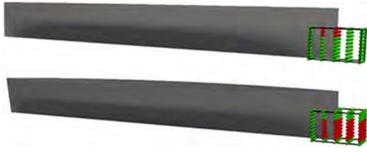
Fig. 22. Two lattices for generating a bulbous bow by FFD method.
