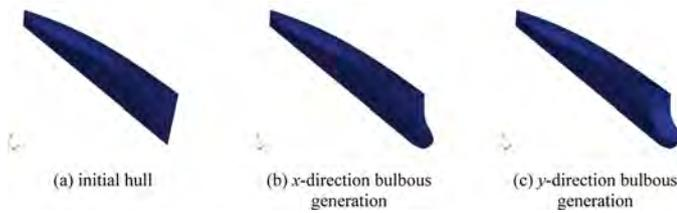
Fig. 31. 3-D view of the generation of a bulbous by RBF method.
