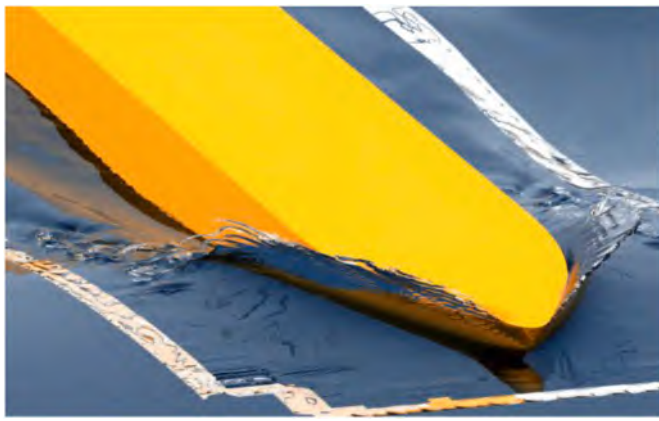
Fig. 11. Instantaneous wave surface of KCS wave breaking at wave crest encounter.
