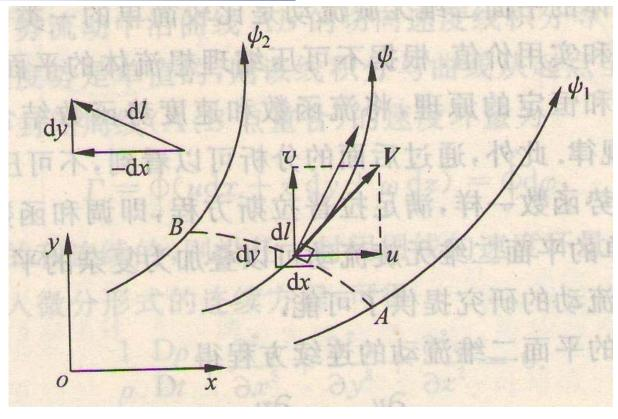
$$q = \int_{A}^{B} v_{n} dl = \int_{A}^{B} \left[ u \cos(n, y) + v \cos(n, x) \right] dl$$
