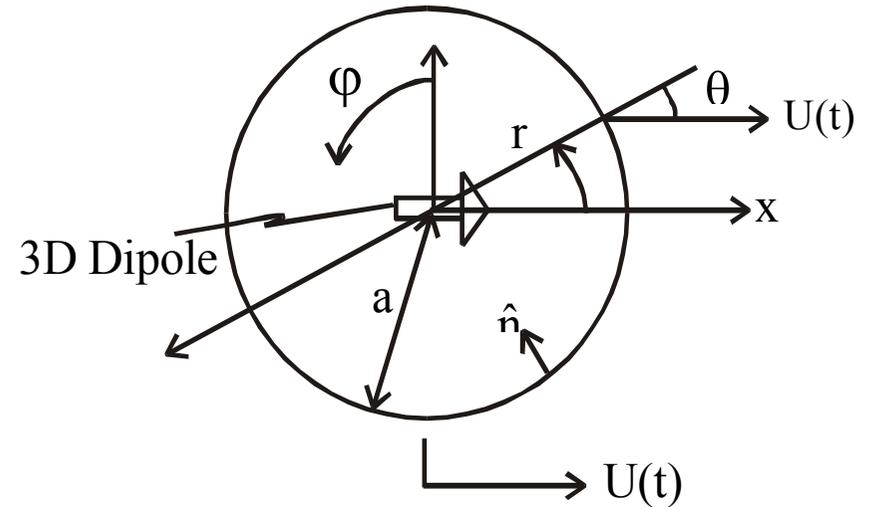
$$\begin{cases} \nabla^2 \phi = 0 \\ \left. \frac{\partial \phi}{\partial r} \right|_{r=a} = \mathbf{U} \cdot \mathbf{n} = U(t) \cos \theta, \quad \text{在球面上} \\ \nabla \phi \rightarrow 0, \quad \text{当 } |\mathbf{x}| \rightarrow \infty, \quad \text{无穷远处条件} \\ \nabla \phi = \mathbf{U}_0, \quad \text{当 } t = 0, \quad \text{初始条件} \end{cases}$$
