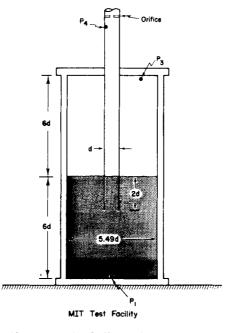
FIG. 12. Schematic of MIT single-vent test apparatus.
