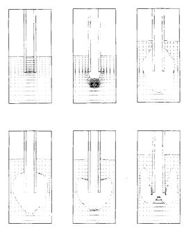
FIG. 13. Velocity vectors and free surface configurations computed when air is forced through submerged vent pipe.
