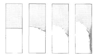
FIG. 10. Evolution of a Rayleigh-Taylor instability started by a pressure perturbation. Times are 0.0, 0.4, 0.8, and 1.6.
