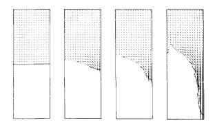
FIG. 11. Repeat of calculation shown in Fig. 10 using pure acceptor cell advection for F. Note the considerably more irregular surface in the last frame.
