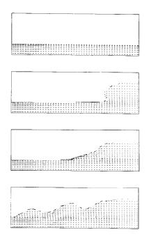
FIG. 9. Velociy vectors and fluid configuration for breaking bore problem at times 0.0, 6.50, 8.51, and 14.01.
