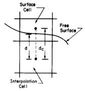
FIG. 4. Sketch showing definition of quantities used in defining free surface pressure boundary condition.
