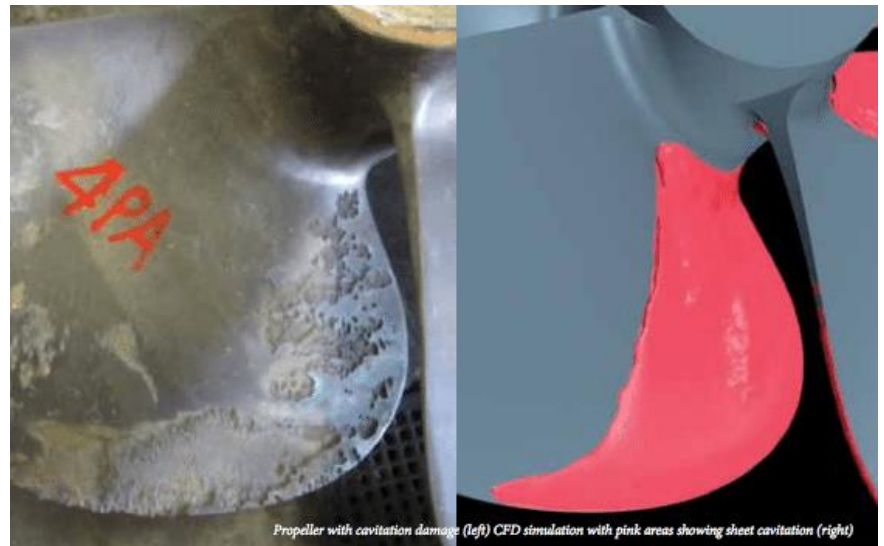
Propeller with cavitation damage (left) CFD simulation with pink areas showing sheet cavitation (right)
