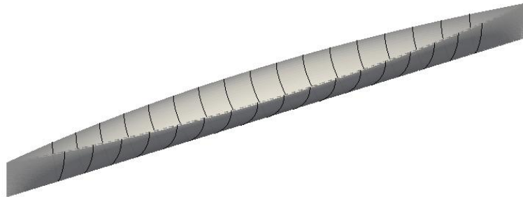
图 4-2 Wigley 水下切片示意图 Fig.4-2 the sections of Wigley under waterline
