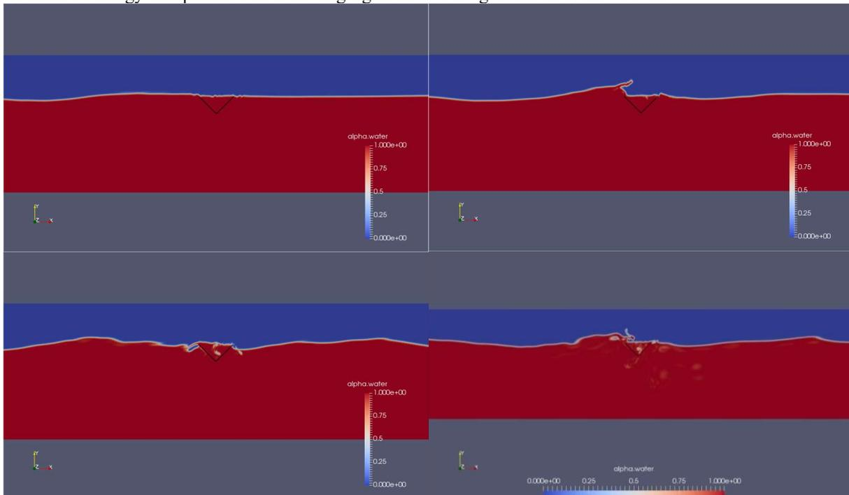
**Figure 2: wave propagation between the two plates**
