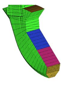
Figure 1: The geometry of the chute
