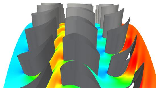
Figure 5: Aachen test case geometry and velocity field.
