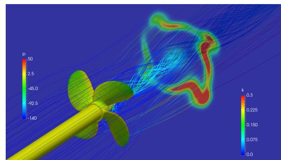
Figure 3: A ship propeller simulation results.
