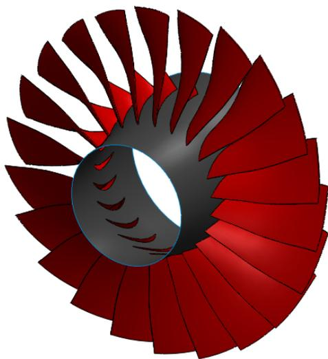
Figure 4: NASA rotor 67 geometry, full annulus.
