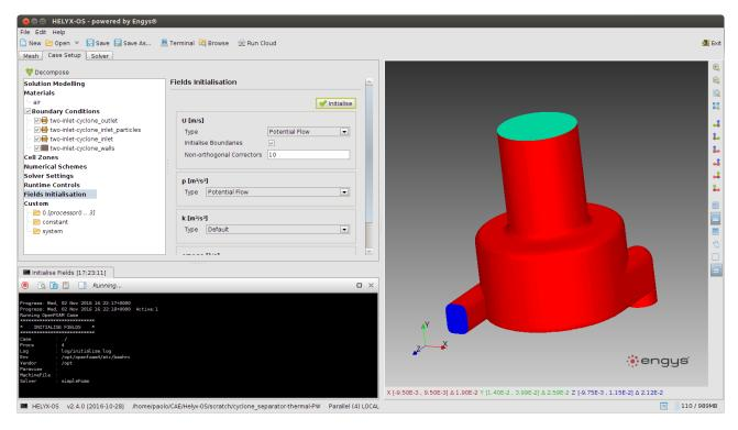
Figure 1 – HELYX-OS graphical user interface for OpenFOAM®
