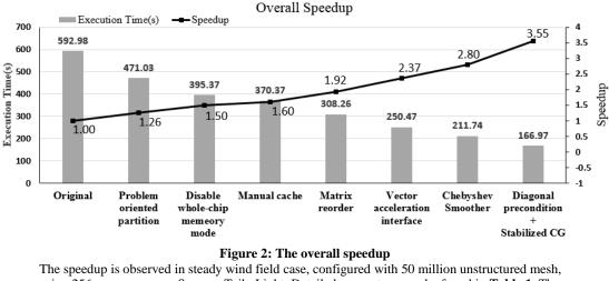
The speedup is observed in steady wind field case, configured with 50 million unstructured mesh, using 256 core groups on Sunway TaihuLight. Detailed case setups can be found in **Table 1**. The pillars illustrate the "Execution Time" reported by OpenFOAM after 40 SIMPLE iterations. Effects are accumulated. The solid line shows the speedup converted from the "Execution Time" result.
