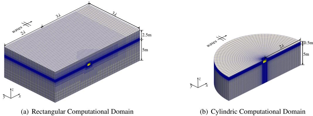
**Figure 4: Mesh configuration for the test case**
