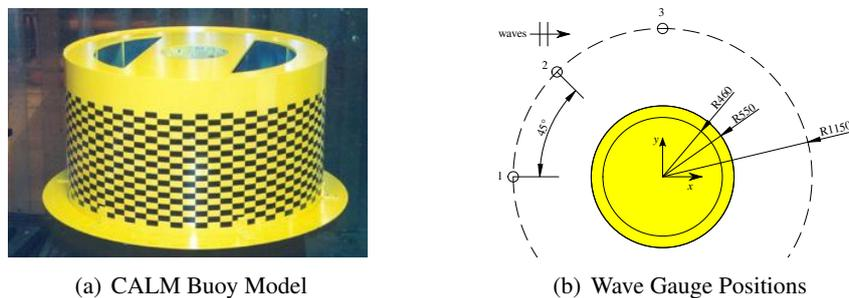
Figure 3: Experiment setup for CALM buoy in waves
