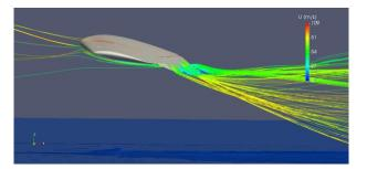
Fig. 2 Streamline passing through flaps at AoA=5 degree
