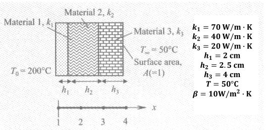
This is a problem with discontinuous data (ICONT=0) because a=kA is discontinuous (as well as h1/=h2/=h3). Consider a 3-element (nonuniform) mesh of linear elements
