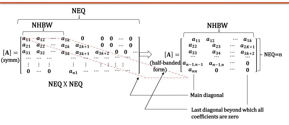
The upper diagonals (parallel to the main diagonal) take the position of respective columns in the banded matrix. Thus, the banded matrix has dimension NEQ X NHBW, where NEQ denotes the total number of equations in the problem
