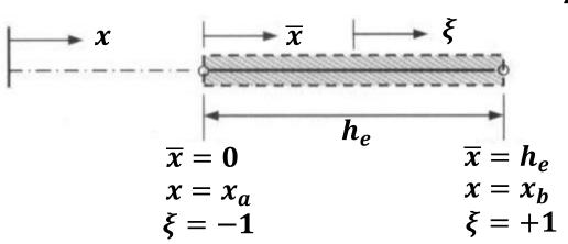
local coordinate ξ is called the normal coordinate or natural coordinate, and its values always lie between -1 and 1, with its origin at the center of the element
